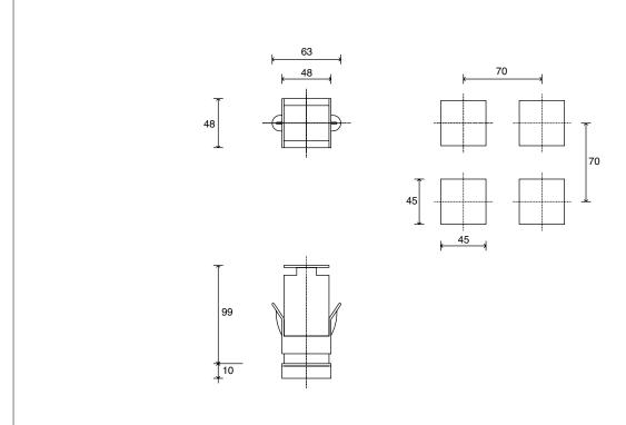
Dimensions: 48x48mm (1/16 DIN) depth 99mm
