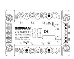
L1: Phase 1 input L2: Phase 2 input L3: Phase 3 input T1: Phase 1 output T2: Phase 2 output T3: Phase 3 output Control signal (AC) A1: Control signal (AC) A2: B1: Alarm output (option) R2· Alarm output (option) Led ON: Red led signal indicator
