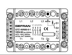
L1: Phase 1 input L2: Phase 2 input L3: Phase 3 input T1: Phase 1 output T2: Phase 2 output T3: Phase 3 output A1: Control signal (+) A2: Control signal (-) B1: Alarm output (option) B2: Alarm output (option) Led ON: Red led signal indicator
