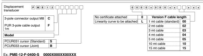
PME 12 displacement transducer, cable output, useful electrical stroke (C.E.U.) 400 mm, PCUR031 cursor, no certificate attached, cable length 1 m.
