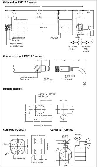
Important: All the data reported in the catalogue linearity and temperature coefficients are valid for sensor utilization as a ratiometric device with a max. current across the cursor circuit Ic  $\leq 0.1~\mu$ A.
